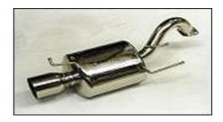
Advanced Vehicle Operations - AVO - were one of the first companies in Australia to offer a 3-inch system to suit the WRX. Their current off-the-turbo system uses stainless steel 3-inch mandrel piping, a modified standard cat (or the choice of a US aftermarket item), high-flow pre-silencer and a polished rear muffler with the choice of either a 3½- or 4-inch tip. This simple bolt-on system also complies with noise and emission requirements. Tried and tested.
