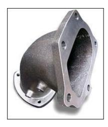
Again - getting a little more extreme - APS also have a High Flow Turbo Discharge Housing. This housing is designed to deliver optimum gas flow and the ability to cope with sky-high EGTs. It is made from high temp ductile iron and is available to bolt directly onto TD04, VF22, VF23, VF24 and VF28 IHI turbochargers (as fitted to MY97 - 00 WRX, STi 2-door Version 5 and STi 4-door Version 6).
