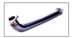
The A'PEXi GT-spec system is a more street-legal system, using the same N-1 series exhaust configuration (with its minimal number of bends). The rear box is again made from that wonderful SUS304 stainless steel, while an additional stainless steel centre muffler allows the system to meet most street-legal requirements. Like all A'PEXi WRX systems, this is a cat-back unit only.
