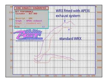
Originating from Japan, **A'PEXi** exhaust systems are amongst the very best on the market. You only need to consider that - it's claimed - many car companies rely on A'PEXi quality to produce their own OEM exhaust systems. Robotic TIG welds are used, all canisters use aircraft quality SUS304 stainless steel and the pipes are protected by a titanium particle based high temperature paint. Note that these systems are all sold as cat-back - you'll need to find your own dump pipe...
