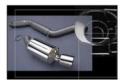
You can trust **TRUST**...Imported from Japan, the BL Extreme cat-back only systems are street-legal and feature a highly polished high-grade stainless steel muffler. Optimum sized mandrel bent piping is utilised and exhaust flow is maintained with straight-through design rear box. With a diameter of 80mm, this system suits all MY WRXs.
