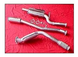
The workshop of **MRT** offers three stages of exhaust upgrades for the WRX. Replacement of the rear muffler only, a new exhaust from the turbo-back, or a total upgrade from the engine-back. MRT's overall focus has been on maximum power - but with a good, muted sound. "The note without the headache" as they put it.
