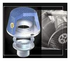
Japanese brand – **GRACER** – has the Airinx air filter to delivered minimal airflow restriction together with claimed improved filtration. The Airinx features a solid wire mesh for the shell and a lightweight ABS inner funnel. A urethane foam filter element is used to protect your turbo and engine. Can be bought for any model WRX.
