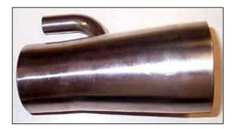
Ever noticed that early (MY94 - 97) WRXs are equipped with a plastic resonant chamber located between the aiflow meter and the compressor inlet? This plastic box primarily serves to give a smooth idle quality - but it's also the cause of a minor airflow restriction. **Possum Bourne Motorsport** sell this replacement pipe to slide straight into the place of that darn resonant chamber.
