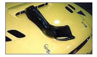
Vin Macaro of **BGT** is proud to offer this intake kit to upgrade the airbox on all MY97-on WRXs. Sucking air from the car's under-pan airflow, BGT have kept the intake air temps low while also providing increased flow into the airbox. A water escape is also incorporated into the duct to lessen the likelihood of water entering the intake. BGT also offer the choice of a KNor A'PEXi panel-type air filter to fit right in.
