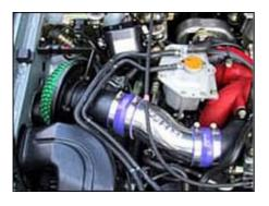
The ultimate HKS air intake - however - is the newly-released Racing Suction Kit. Here, the WRX's standard rubber intake pipe is replaced by a gas-flowed metal substitute - which means there's less restriction further down the intake system. All pipework and mounting hardware is included in this particular kit - which is suited only to MY97-on.
