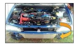
For those chasing absolute minimal intercooler pressure drops and maximum charge-air cooling, the AVO front-mount 'cooler is right up your alley. Again, featuring bar-and-plate core design, the front-mount performs well up to expectations and comes together with HPC'd steel intercooler piping and high pressure/high temperature hoses. This front-mount core is available to suit MY97 - 99 WRXs.
