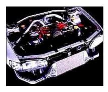
The more serious BPM front-mount air-to-air intercooler gives even further improved heat dissipation characteristics, as well as less pressure drop. Sold as a kit - complete with all necessary piping - this core uses all the space in front of the radiator while also freeing up space in the engine bay for a monster turbocharger... Both top and front-mounts are available to suit all models.
