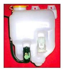
The tank and pressure components of the water spray system can be configured in various ways. MRT have this elegant twin pump replacement washer bottle (one pump is dedicated to the intercooler spray), which screws straight in for a totally stealth installation. Alternatively, separate windscreen washer-type pumps are also available for a DIY set-up.
