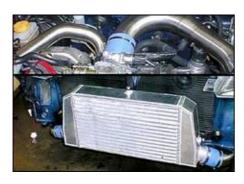
A front-mount intercooler kit is also sold alongside the top-mount. Using a 450mm x 250 x 90mm bar-and-plate core with alloy plate end-tanks, it comes beautifully assembled with stainless TIG welding and silicone high pressure joints.
